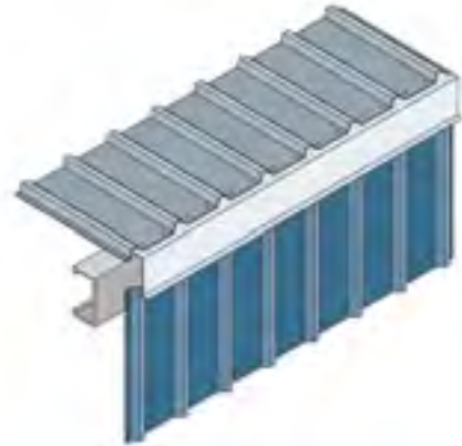
Eave Trim Oversized architectural trim combines with roof and wall closures.
